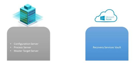
When setting up your environment, you will need to consider the setup on both Azure and on-premises sides. You will need to build an Azure Site Recovery (Recovery Services Vault) in Azure. You will also need to build a Configuration Server with appropriate configurations on-premises.
